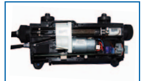
Renault EPB Controller & Motor EPB controller with integral ECU for operating electronically controlled Hand (park) Brake
